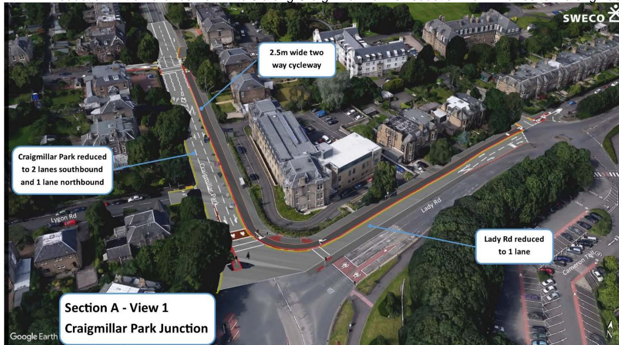
Figure 2.2-View 1, Craigmillar Park / Lady Road / Esslemont Rd / Liberton Rd Junction
